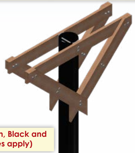
FRP Shear washer that is to be sandwiched between the wood or FRP braces and stringers and used as a washer on the backside of the connection.
