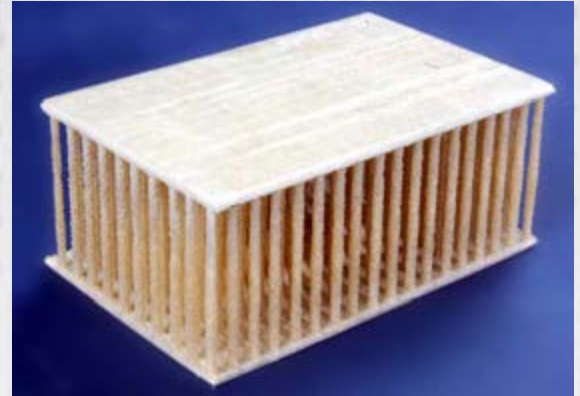
Close Up of the Fiber Insertions with the Core Foam Removed
