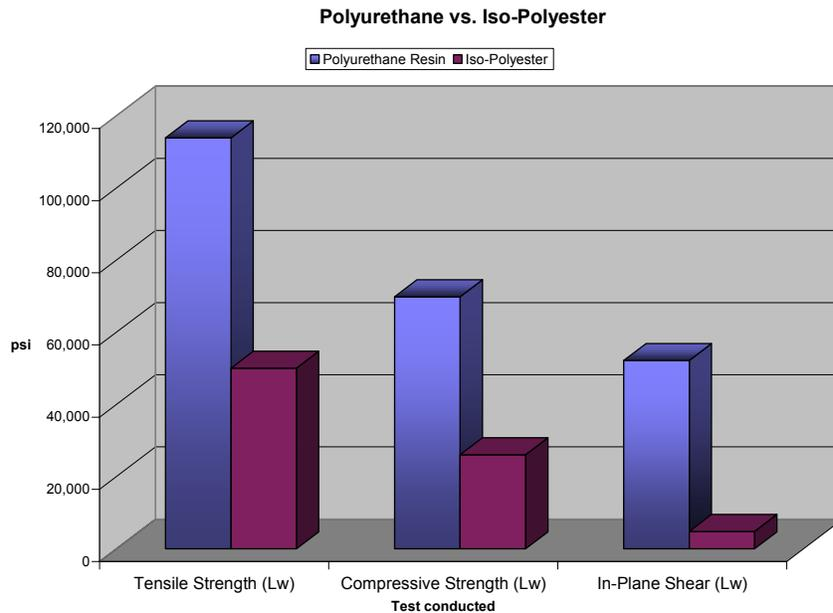
Figure 2.0 Lengthwise mechanical properties
