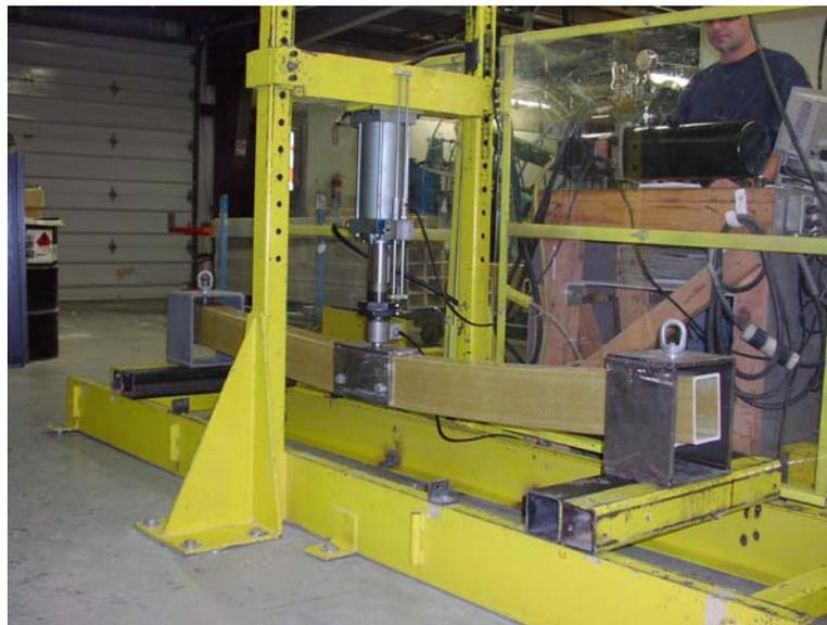
Figure 4.0 Full section bend test
