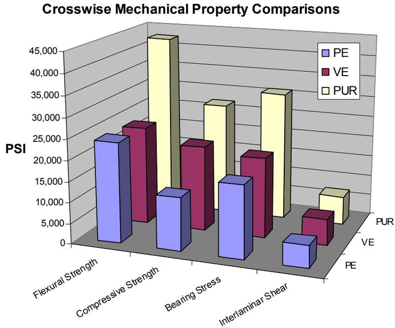
Figure 1.0 Crosswise mechanical property comparison
