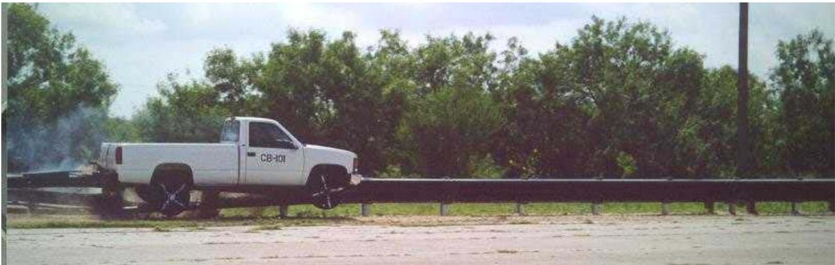
Figure 5.0 ¾ Ton Pickup traveling at 62 Mph; Impact angle 25°
