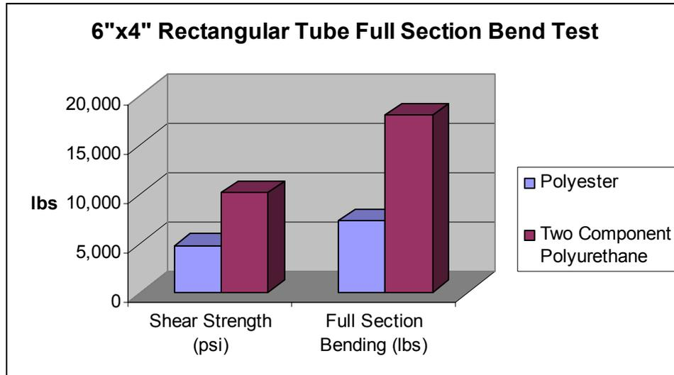
Figure 3.0 Full section bending strength graph
