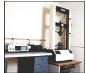
Instron tensile tester produces strength and modulus results
