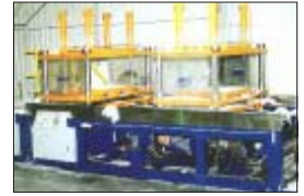
Reciprocating pultrusion machine offers 22" x 60" maximum envelope capacity
